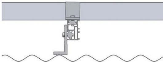
Cross-section of the system showing how the Z-module connection works between interface, rail and clamp.
